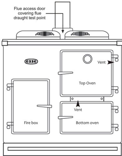
Fig.3a – Flue Damper and Flue Box Door
