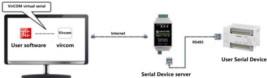
Figure 12 Application example of virtual serial port
