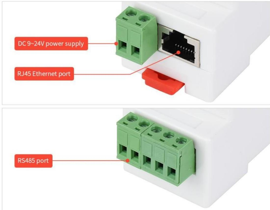
Figure 4 Power supply, network port
